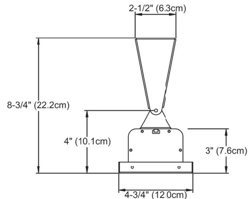
Heater must be installed with the quartz tube horizontally level. For maximum tube life, use a level to find the optimum position for the heater's body. Always maintain the minimum clearances from the heater body to any combustible materials.
