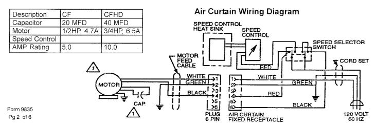
Verify that the power supply matches the electrical requirements of the unit as listed on the data plate on the unit Disconnect power before installing or servicing the air curtain. If the main disconnect is not in sight of the unit, lock it off and tag it to prevent someone from accidentally turning it on Failure to follow these instructions could result in fatal electric shock.
